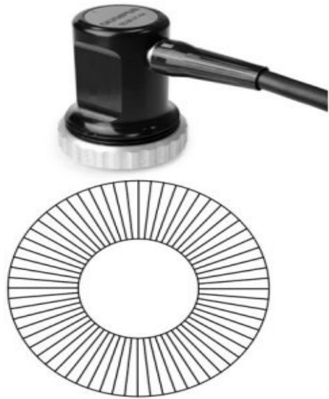
Figure 2. The custom 5D26-12-64 ring-array probe (top) and element distribution schema (bottom)
